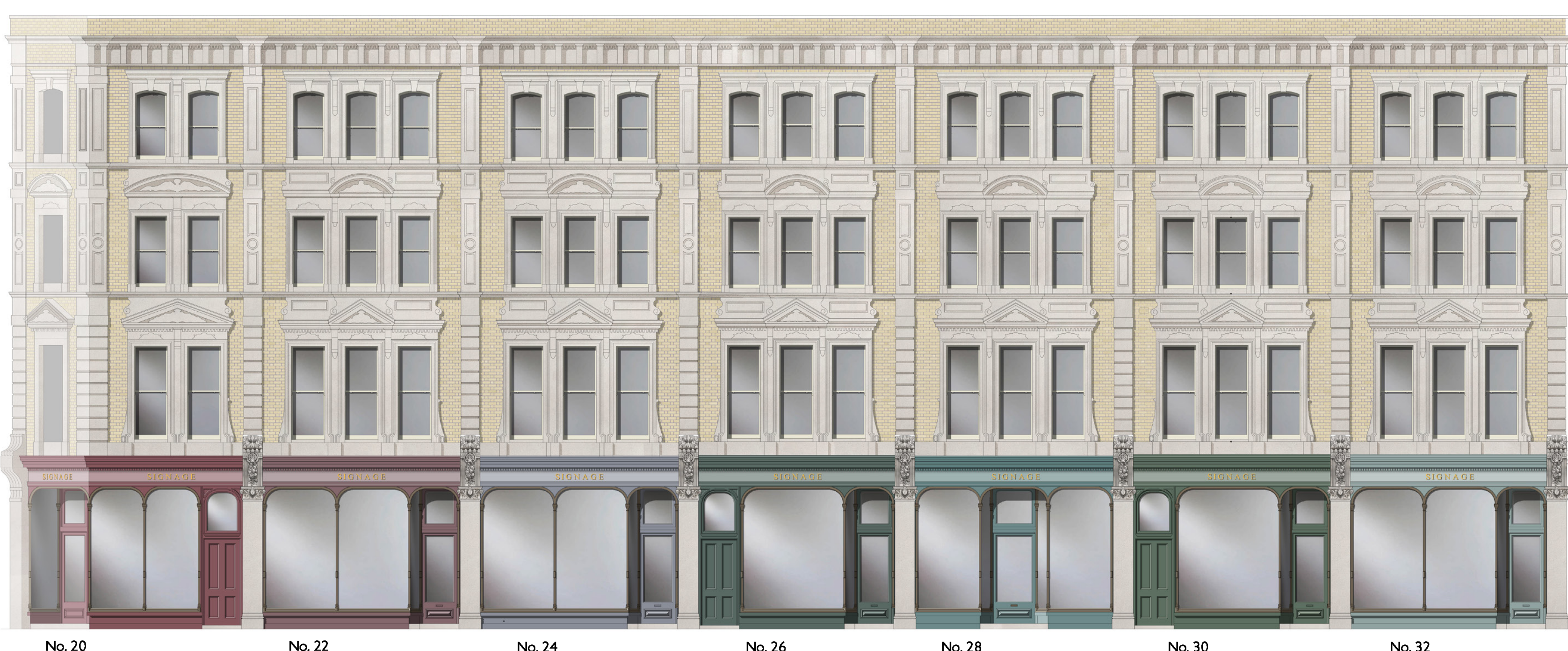
Proposed elevation drawing of Nos 20-32 Thurloe Street showing the proposed new shopfronts
